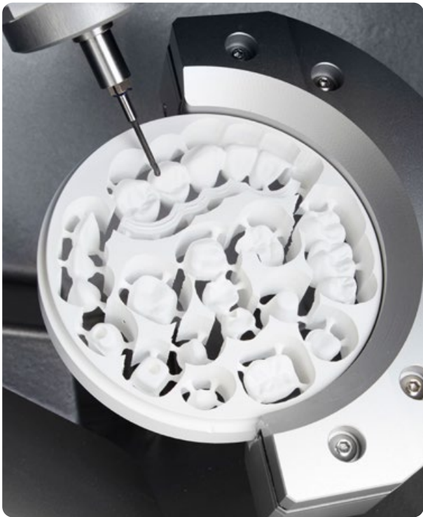
The R5 tilts the spindle (B-axis) by up to ± 35°. This means that the blank holder only needs one moving axis (A-axis), thereby making the entire system more stable.
