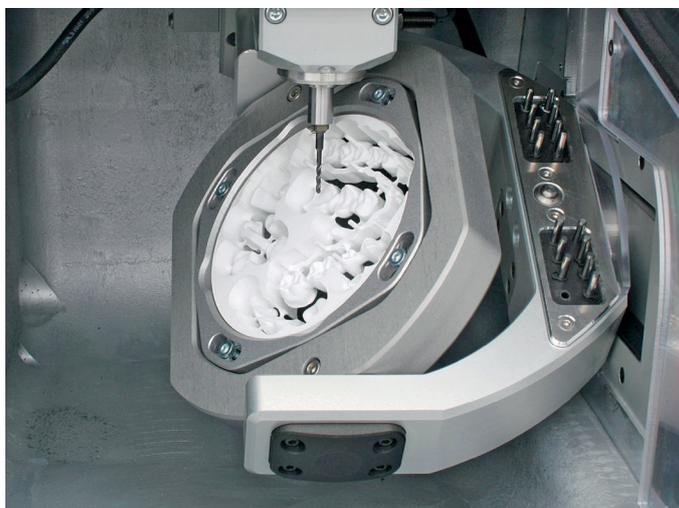
The interior of a vhf S1 during machining. The five-axis milling machine was used to produce the prosthesis samples for the study.
