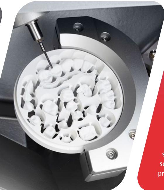
Full range of materials and indications – even with manual blank changing. **directclean** Technology comes standard and, thanks to its smart work area drying system, lets you switch seamlessly between wet and dry processing.
