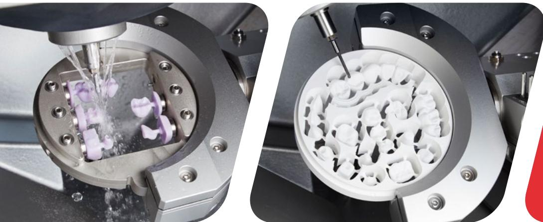
Full range of materials and indications – even with manual blank changing. **directclean** Technology comes standard and, thanks to its smart work area drying system, lets you switch seamlessly between wet and dry processing.
