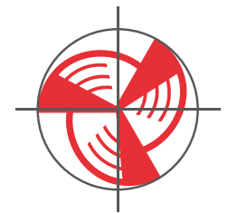
Cross-section of triple tooth cutter: Three cutting edges need much more space.
