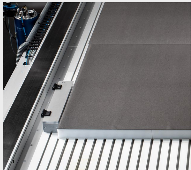
The vhf vacuum fleece not only ensures a fine distribution of the air sucked in through the hole grid, but also serves as outlet material for the milling cutter.
