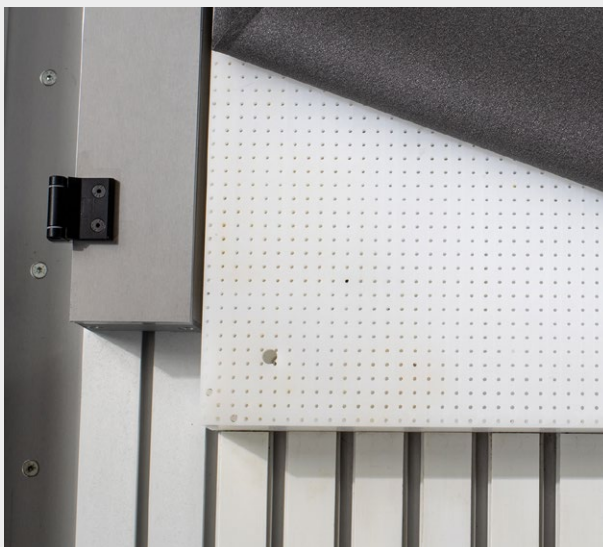
The vacuum elements with a hole grid are fixed on a T-slot table.
